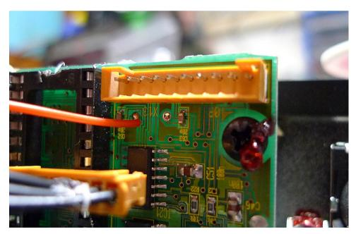
Now you need to solder the wires from the switch to the two terminals on the Behringulizer 2000 PCB where it says 'MODE SWITCH', and the wires from the pot to where it says 'CLOCK POT', as shown in the photo at the top of the next page.
