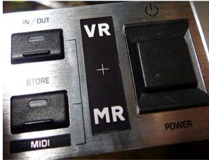
You can now drill the holes for the switch and the reclocking knob. We'd advise using a very small drill bit to drill a pilot hole in the exact centre of the positioning crosses, and then use a 6mm drill bit for the switch and a 7mm one for the reclocking pot. Be careful to get the hole for the pot as central as possible and try not to mess up the stickers by drilling wildly.
