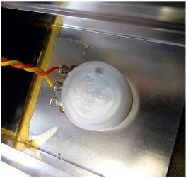
Now you've installed the switch you can solder wires long enough to reach back to the EPROM socket plus an extra couple of cm, to the reclocking pot. You should use the middle and right hand tags, as shown in the image on the previous page.
