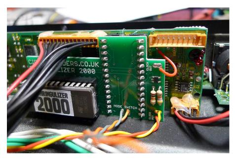
Now just solder the wire coming from where you removed the crystal to the 'CLOCK OUT' terminal on the Behringulizer board, as shown above. Remember to reconnect any of the orange connector blocks you removed during installation and you're finished.
