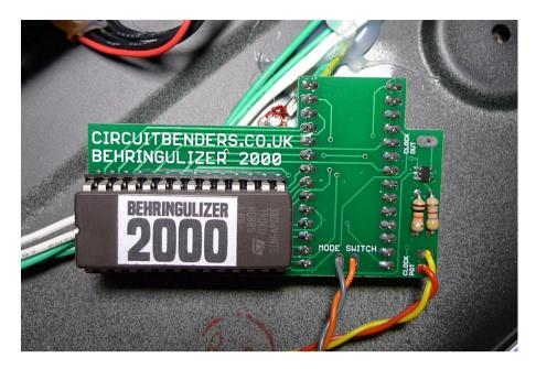
Make sure none of the pins on the other side of the board is bent to the side, then carefully align them with the EPROM socket on the main board and push the Behringulizer 2000 PCB into place as shown below. There shouldn't be any resistance, although on some units there may be some slight friction between the Behringulizer board and the bottom of the casing.
