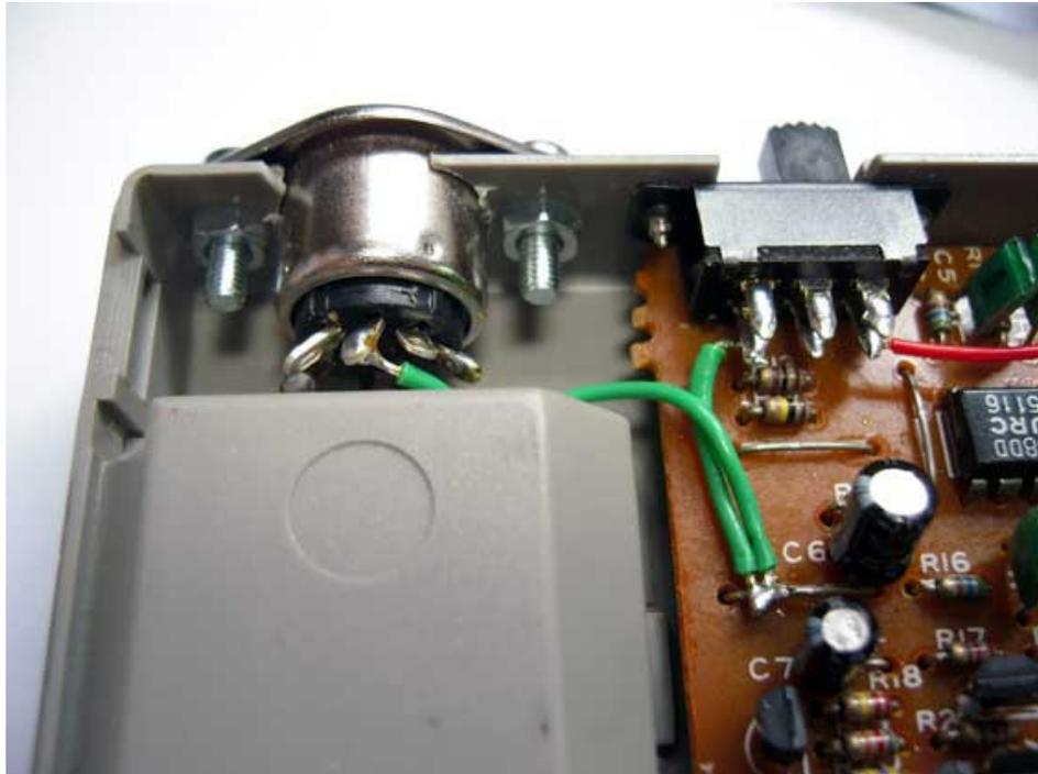
The bottom right hand pin of the switch should be soldered to a 5v source. The most convenient is pin 14 of the IC shown in the image below. Try not to overheat the IC while doing this.
