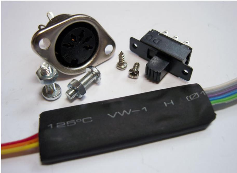
You should have a 5 pin DIN socket with two fixing bolts, a sliding switch with two fixing screws, and the DIN sync interface with the external wiring already soldered onto the board as shown.
